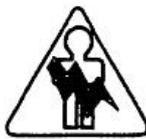
The lightning flash with the arrowhead symbol superimposed across a graphical representation of a person, within an equilateral triangle, is intended to alert the user to the presence of uninsulated "dangerous voltage" within the product's enclosure; that may be of sufficient magnitude to constitute a risk of electric shock.
